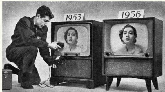
**ELECTRONIC LIGHT METER** recently tested two TV sets equipped with ordinary tubes, with studio camera focused on still picture for uniformity. Proved up to 60% of the brightness and 50% of picture contrast were lost on the 1953 TV set.
